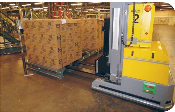
AT WORK CONTROLLING THE AGV TO PICK UP BOXES
